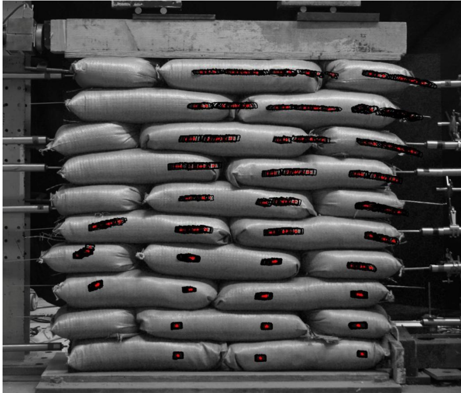
Figure 39 Result of photogrammetric analysis for 'barbwire' with average total normal load of 1.44kN (cycle 1 on graph below)
