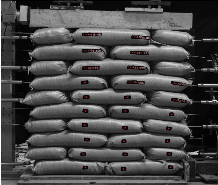
Figure 36 Result of photogrammetric analysis for 'plain' with average total normal load of 0.85kN (cycle 1 on graph below)
