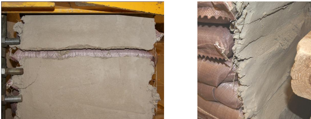
Figure 27 Tensile crack (left) and compression cracking (right)
