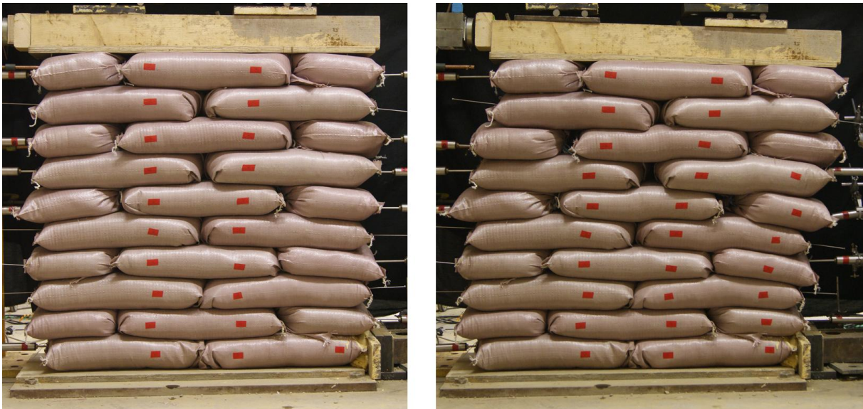
Figure 34 Initial shape (left) and final shape (right) for ‘plain’ model test cycle 4
