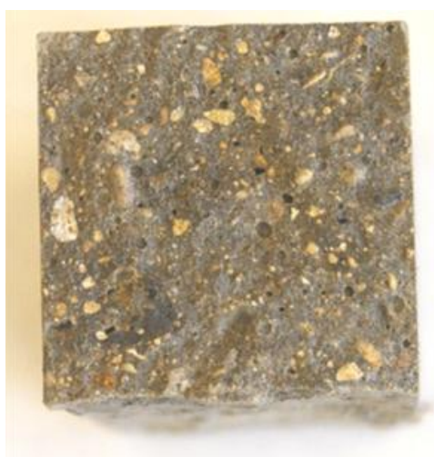
Figure 45 Typical cross section of render prism used in flexural test
