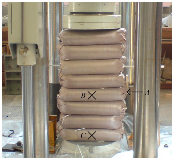
Figure 5.4: 8-bag earthbag stack, with displacement transducer locations indicated.
