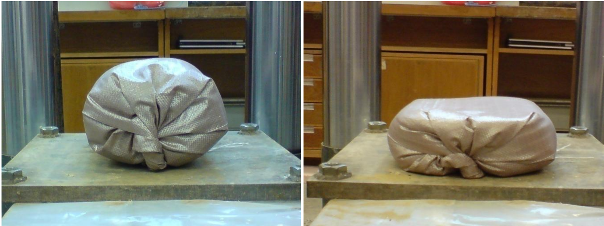
Figure 5.3: Earthbag on testing rig before and after tamping.
