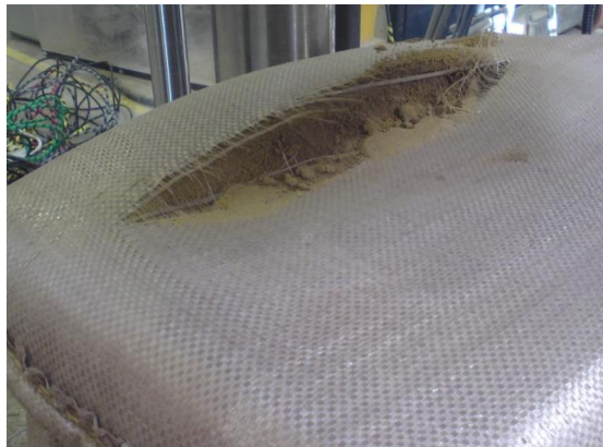
Figure 5.8: Bag tearing of unstabilised 8-bag stack compression test.
