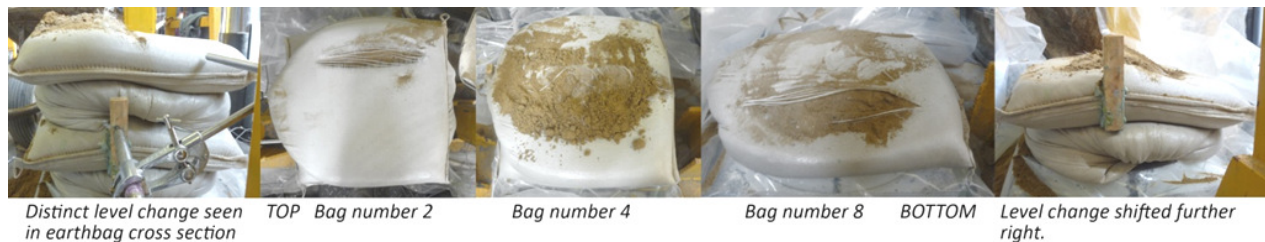
Figure 22: Tearing of 70gsm polypropylene earthbags after compression test
