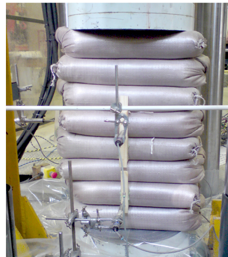
Figure 12: Arrangement for eight earthbag stack compression tests
