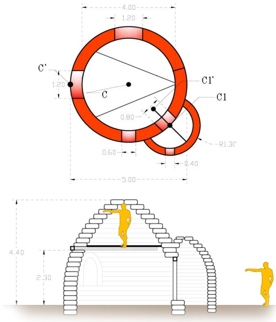
Figure 1: Plan and section of earth bag model
