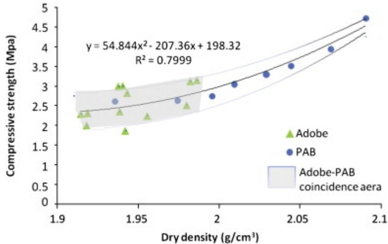
Figure 6: Relationship between ovens dried density and compressive strength (Kouakou 2009)
